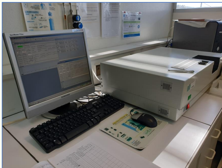
Figure 3 Advanced Mercury Analyser burns the sample to quantify total Hg concentrations in each feather
